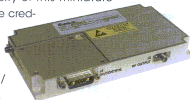
This amplifier module includes control circuitry and GaN devices with capability of providing 50 W output power from 6 to 18 GHz.
